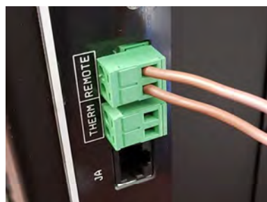
Figure 45 ñ Remote connection
