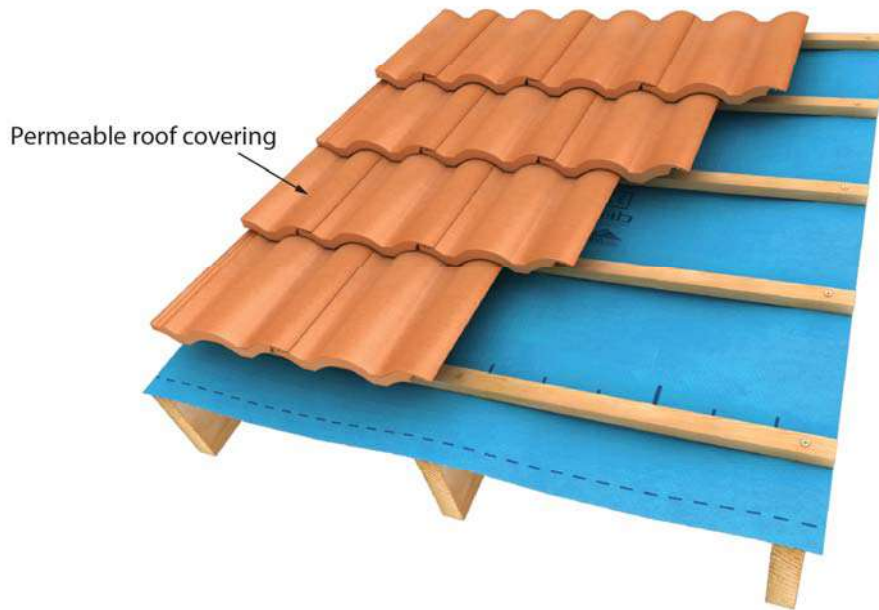
Figure 1: Cold Roof detail with permeable roof covering
