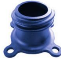
Series 29 B Fire Hydrant Outlet Stainless Steel Outlet 2 1/2" RT Epoxy Coated BSEN10088 W1.4021 M12: 290801311
